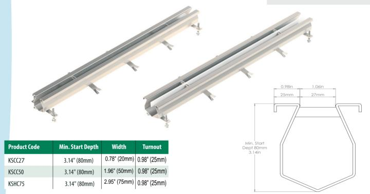
Specify: Kent Super Clean Channel KSCC27; <u>mm</u> length <u>with Ce</u>ntral Trapped <u>Gully</u> outlet; Grade <u>304</u> Stainless steel.
