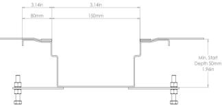
Specify: Kent Vinyl Box Channel KVBC200; to take 200mm wide grating; \_\_\_mm length with Central Gully Outlet KV285/160/110; Grade 304 Stainless Steel; Load Class A.
